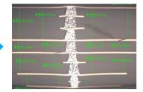
One-time stacking lamination + conductive paste process
