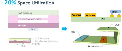
Bending freely to fit mechanical space requirements
