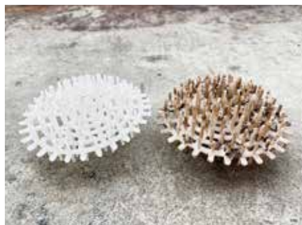
洗滌塔濾材清洗
