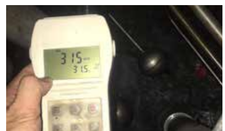
Conductivity Measurement of Tap Water
