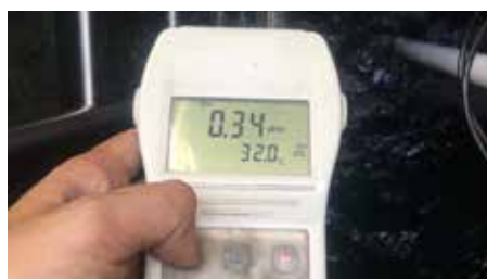
Conductivity Measurement of Pure Water
