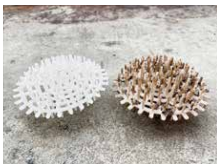
Cleaning scrubber tower filters
