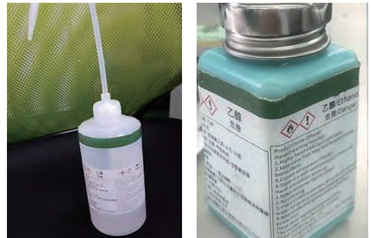
Replacing wash bottles with liquid dispenser pumps to reduce alcohol usage and VOC emissions
