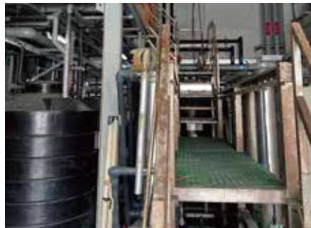
Electrolytic copper recovery system
