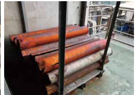
Copper pillars produced from the electrolytic copper recovery system
